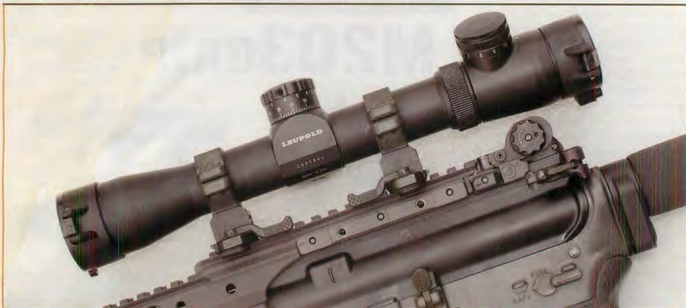
The Leupold MR/T is an exact copy of the SF TS30-A2 Sniper Scope used on the SPR. It is mounted with A.R.M.S. #17 ThrowLever rings.
