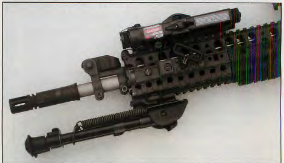
The Harris Bipod, PRI Folding Front Sight and AN-PEQ-2 Laser are SOP on current SPR's. The S.I.R. System and SureFire M556FA Suppressor adapter are new.
